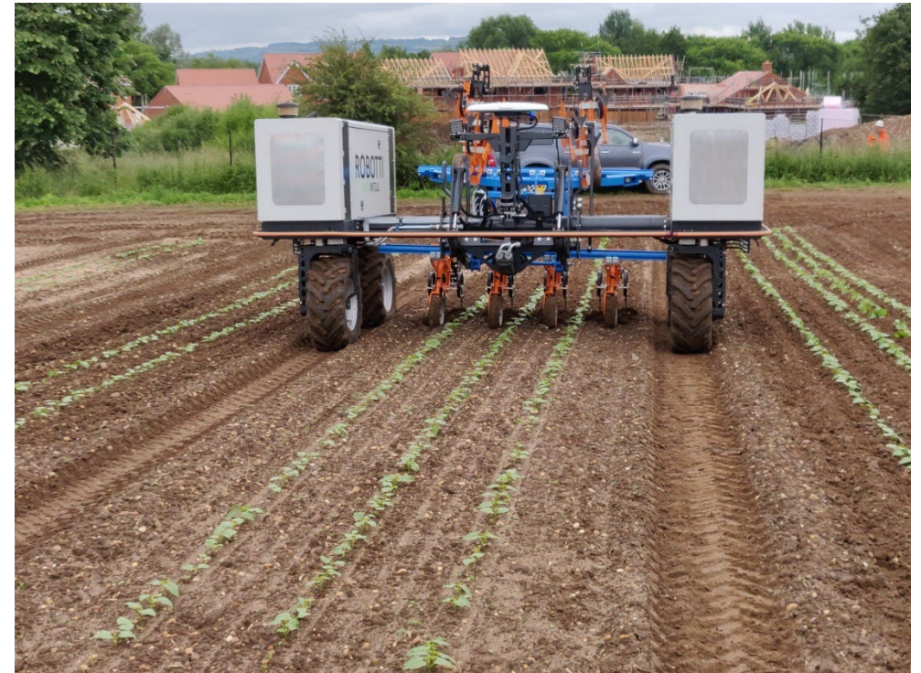
Robotti, weeding robot, weeding French beans on Sandfield Farm, Stratford on Avon, UK, 25 June 2021
